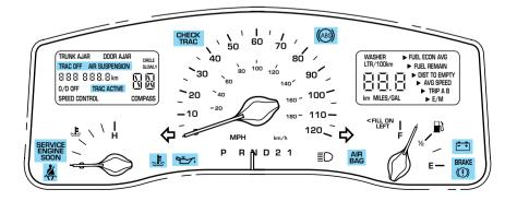
Make sure the corresponding lights illuminate briefly. If a light fails to illuminate, have the vehicle serviced.
